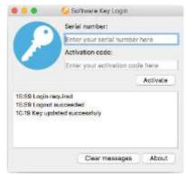
Menu bar. The Icon color will vary, based on its status. To activate the Software key, you must insert the Serial number and the respective Activation code.
