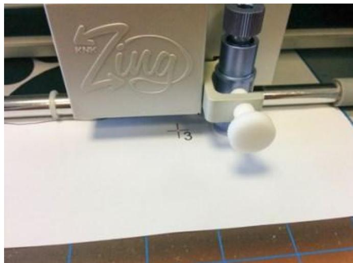
Move to the center of the third point using the arrow keys and press Cut to start the actual cutting process.
