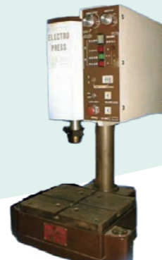
1984 JP-20 Electro Press (servo press) No. 1
