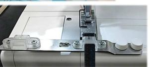
"**Bias Tape Guide**" that can guide bias tape (single fold) and sew it on to knit fabric.
