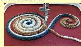
Point 2 The feet are easy to thread, with an open toe and plate design Slide the thread under the plate, and pass it through the presser foot hole. A very user-friendly design!
