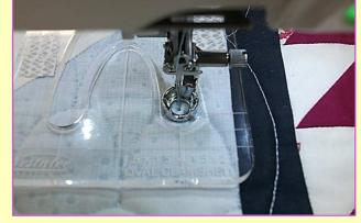
Point 3 Marks on the foot can be used to determine the center point of the foot Marks help to see the center point of the foot hole. This helps to create accurate ruler work designs.
