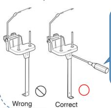
A Phillips screwdriver is required to adjust the spool stand support plate.
