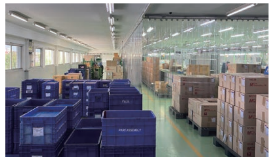
Reduction of electricity consumption by installing curtains Janome Thailand Co., Ltd.
